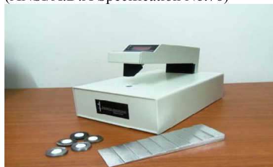
Figure 1. Densitometer, Some specimens, and Aluminum step wedge that were used for Radiopacity test.
